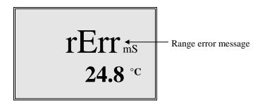
If this happens, simply press and release the [ENTER] key again until a range is selected which is suitable for your sample. If you get lost and don't know if you're in a manual range or autoranging, simply turn the instrument off and back on. The instrument will default to autoranging when first turned on.
