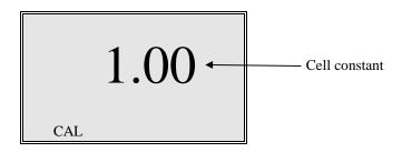
4. Use the [UP ARROW] or [DOWN ARROW] keys to change the value to the desired new cell constant.
