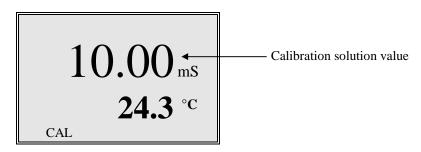
9. Once the display reads the exact value of the calibration solution being used, press the **[ENTER]** key. The word "**SAVE**" will flash across the display for a second indicating that the calibration has been accepted.
