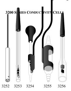
Dip cells are generally used for routine conductivity measurements. The 3254 Fill Cell is designed for small sample or high throughput work. It requires only 5 ml of sample and can make measurements quickly from one sample to the next.
