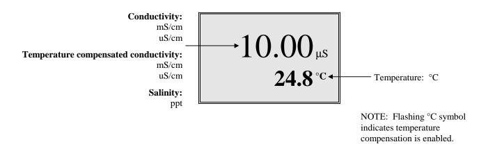
The [Mode] key is used to select the current display mode. Mode choices are conductivity, temperature compensated conductivity or salinity. Temperature is always displayed at the bottom of the screen.
