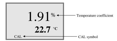
2. Use the [UP ARROW] or [DOWN ARROW] key to change the value to the desired new temperature coefficient.
