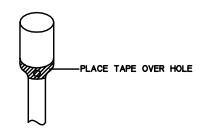
When a dip cell is used as a fill cell, the cell's vent hole is sealed and the electrode chamber is inverted and filled with solution, changing the cell constant (K). The cell will require calibration after being configured as a fill cell.
