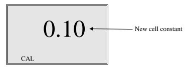
5. Press the [ENTER] key. The word "SAVE" will flash across the display for a second to indicate that your change has been accepted. The 3100 will return to normal operation mode.
