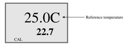
3. Use the [UP ARROW] or [DOWN ARROW] key to change the value to the desired new reference temperature (the allowable range is 15°C to 25°C).
