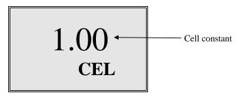
If the instrument detected a problem, the display will show a continuous error message. For a list of these error messages, see chapter 6 *Troubleshooting*. After the instrument completes this diagnostic routine, the following screen should be displayed (with no cell connected).
