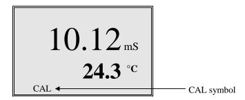
The CAL symbol will appear at the bottom left of the display to indicate that the instrument is now in Calibration mode.
